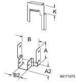
Used to reduce to a smaller size cable tray (right slope shown). **BULLETIN: F23**
